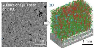
Statistical assessment of various material parameters and implementation in stochastic mesoscale models of SHCC and hybrid fiber reinforced composites
