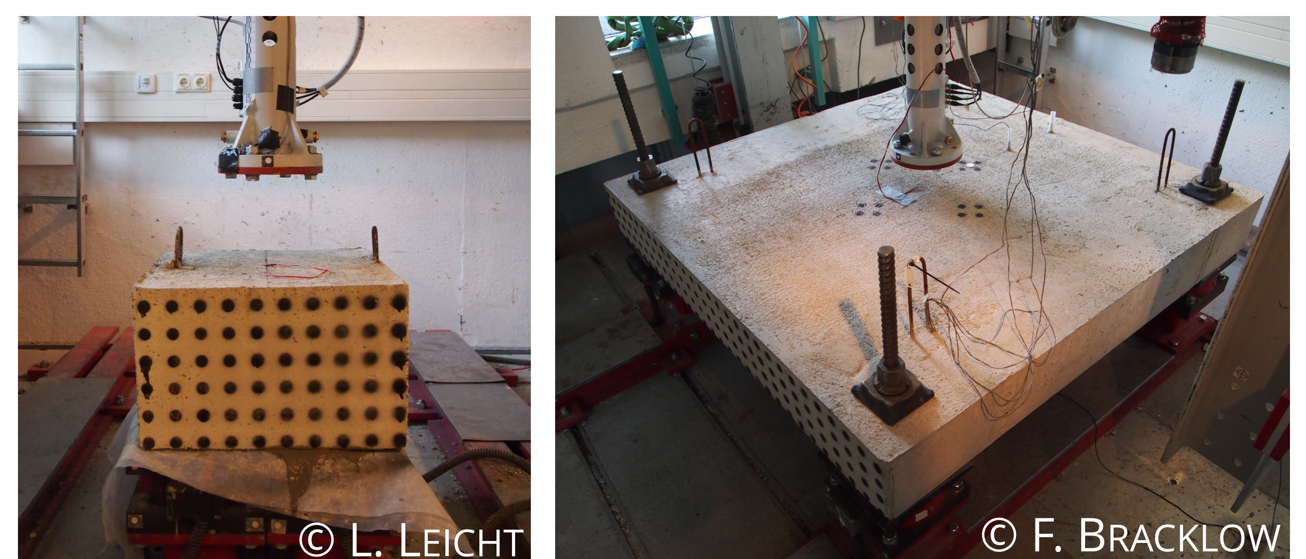
Cuboid (left) and plate (right) testing in the drop tower
