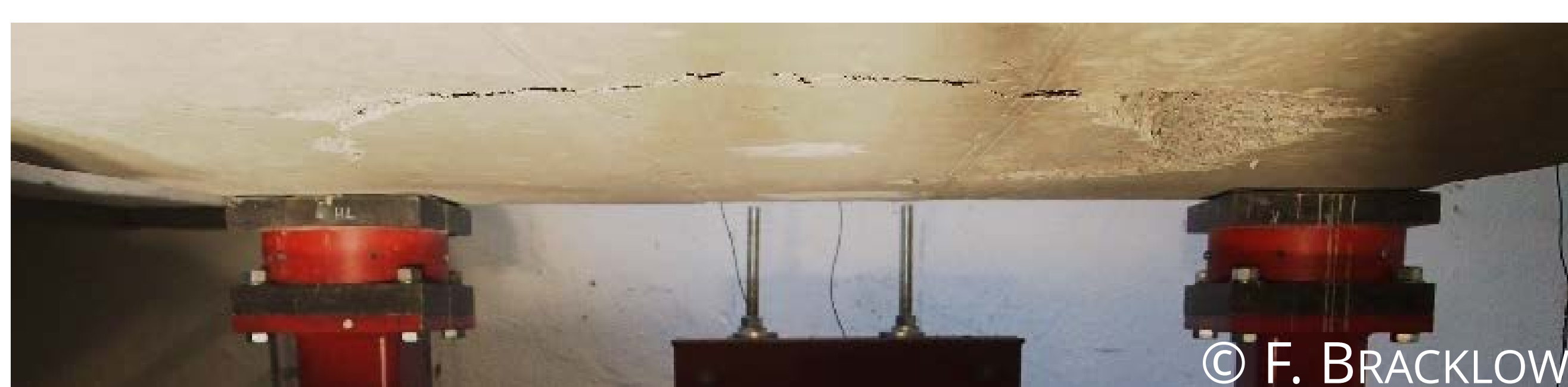
Spalling (top) and scabbing (bottom) damage due to wave propagation in structural members
