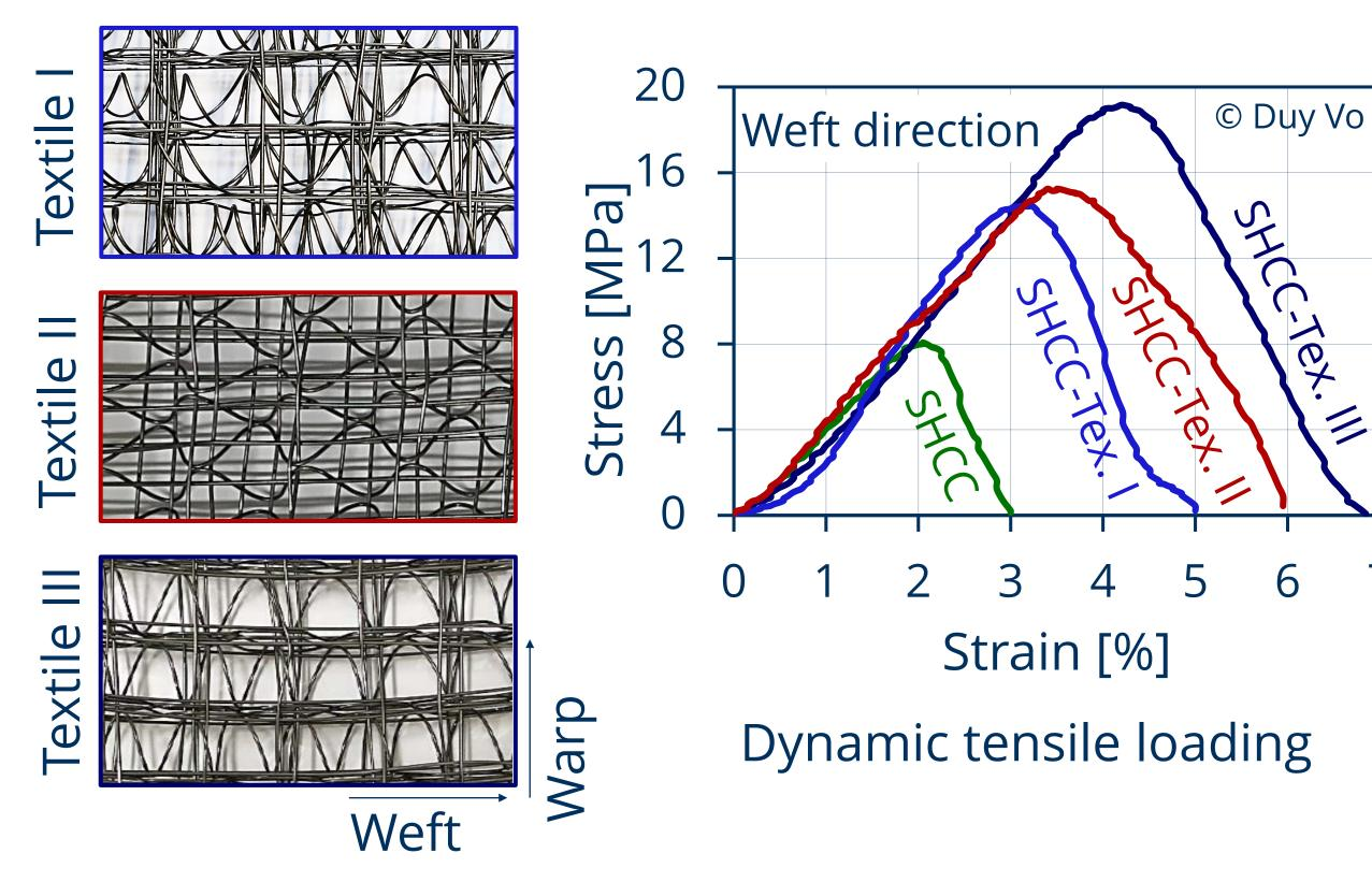
Characterization of the composite structure in drop tower tests and dynamic impact punch tests
